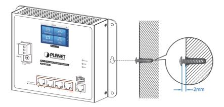
Figure 4-4: Router is hung on the wall
