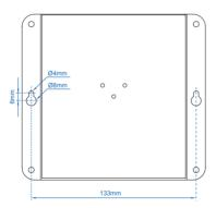
Figure 4-2: Getting mounting holes aligned
