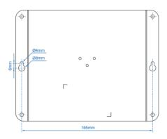
Figure 4-1: Getting mounting holes aligned
