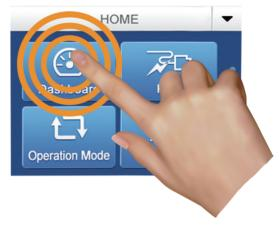
Figure 6-1: To wake the LCD touch screen
